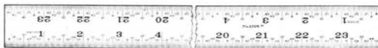
Fig. 4-7d. 12-in. rule. Note how the graduations are numbered. This rule has No. 4 graduations (see table).
