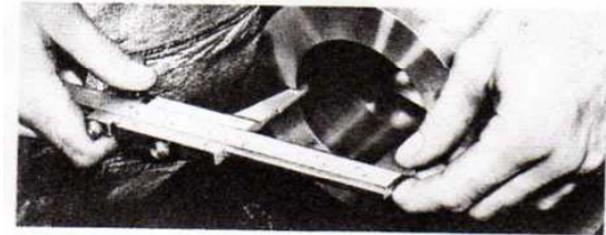
Fig. 4-24. Making an inside measurement with vernier caliper.
