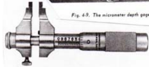
Fig. 4-7. Jaw-type inside micrometer. (Scherer-Tomica)
