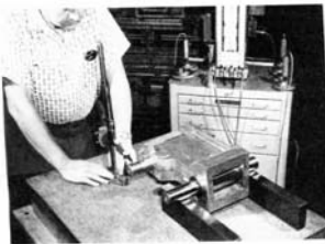
Checking drill press column and quill bearing surfaces for alignment. Note air gage in background - used to check hole diameters.
